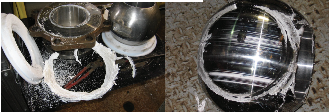
STUCK: SOLIDIFIED MEDIA FOUND IN DIS-ASSEMBLED BALL VALVE, LEADING TO SERVICE INTERRUPTION
